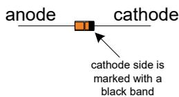
"Reverse polarity of one another" means to connect the cathode of each diode to the anode of the other diode.
