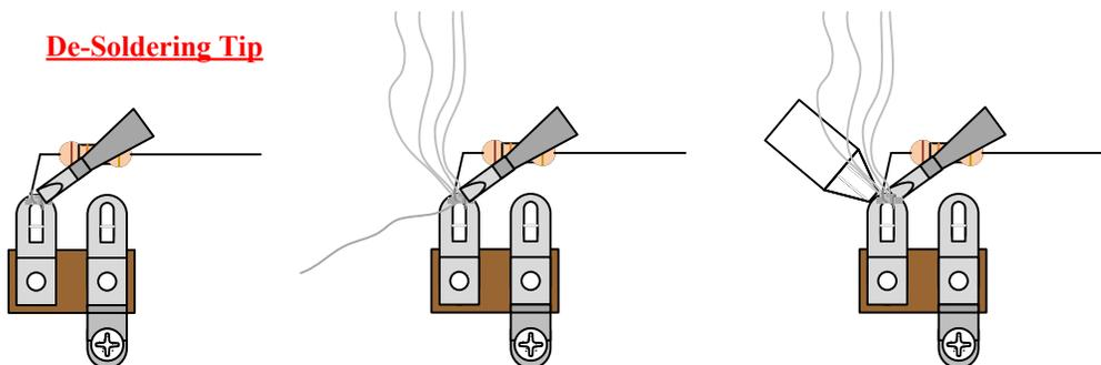
1. Heat up old solder joint with the soldering iron.
